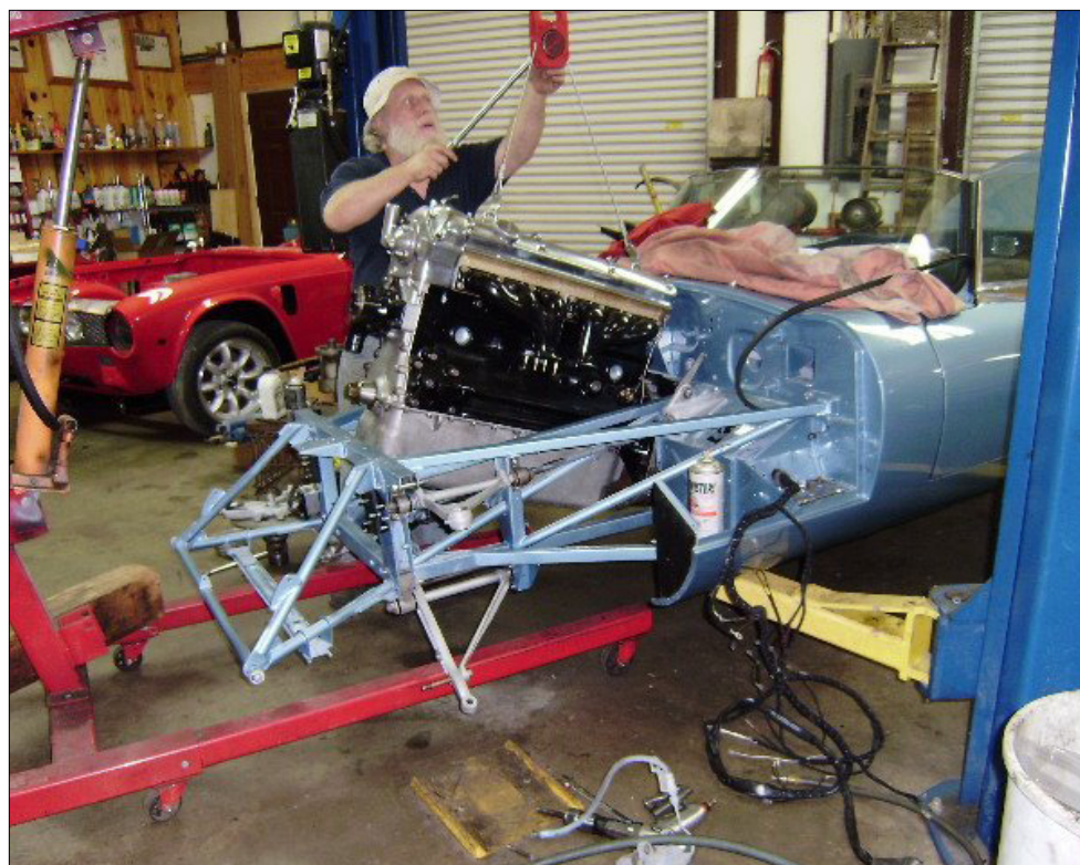
During the process of returning this Jaguar to its original condition, Bart is installing a newly-rebuilt engine into the customer's 1964 XKE.
